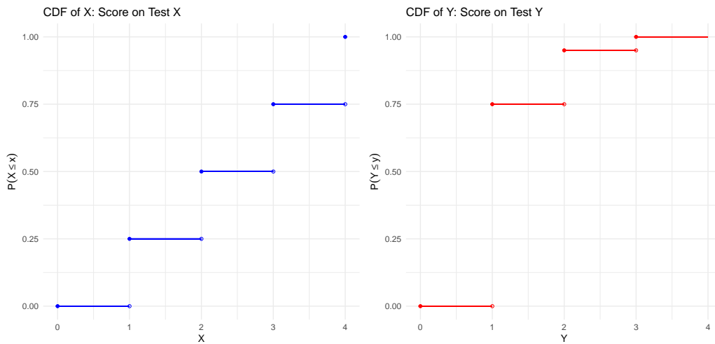
Figure 1: The cumulative distribution functions (CDFs) for the two example tests. We treat the score as a random variable, whose distribution is defined by observed test percentiles. The CDF for a discrete distribution is a right-continuous function defined for all real numbers. The upper limit is 1 and the lower limit is 0.
